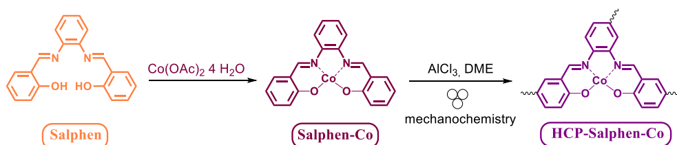
Figure 5.8 Functionalized hyper-crosslinked polymer catalysts to produce 2,5-furan dicarboxylic methyl ester (FDME).
